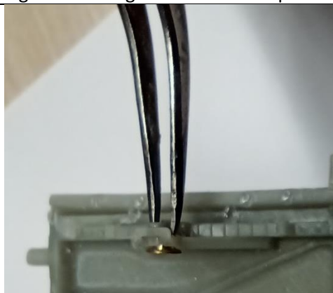
Figuur 11: aslager testen in de aspot
