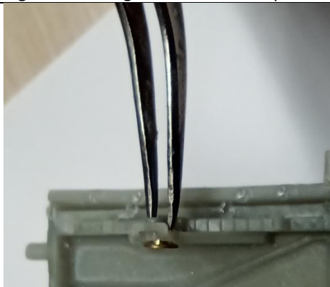
Figuur 11: aslager testen in de aspot
